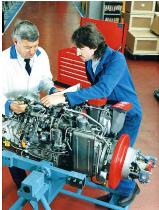
Rolls-Royce Gem aero engine. As well as the main civil engine work, work continued at various Rolls-Royce sites on other engine products. The Gem aero engine was made at the Rolls-Royce Leavesden site near London and powered the Lynx helicopter.
